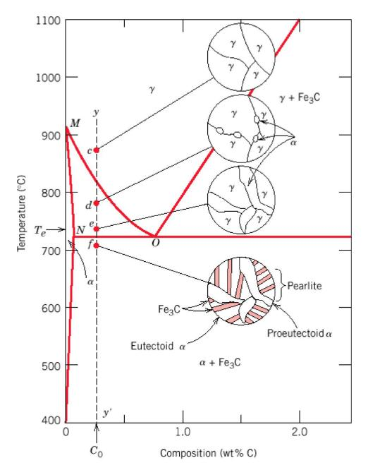
How to calculate the relative amounts of pro-eutectoid phase ( $\alpha$  or Fe3C) and pearlite?
