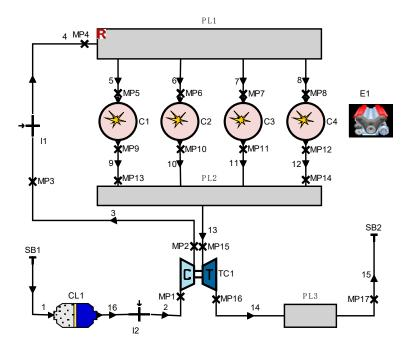
**Figure 10.** The AVL BOOST engine module: I1—water injector; I2—HHO injector; SB1,2—system boundaries; PL1—inlet manifold; PL2—exhaust manifold; PL3—exhaust silencer; CL1—air cleaner; MP1–17—measuring points; C1–4—engine cylinders; 1–15—connection tubes.
