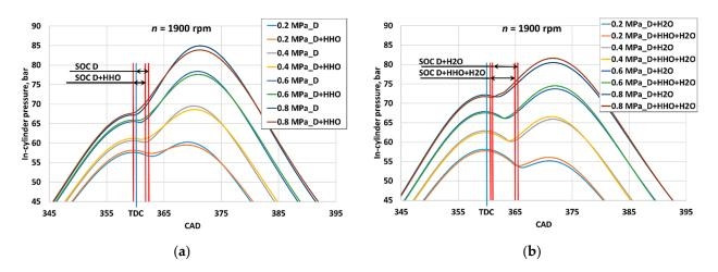
**Figure 11.** In-cylinder pressure vs. CAD for D and D+HHO modes (**a**), D+H<sub>2</sub>O and D+HHO+H<sub>2</sub>O modes at the various *BMEP* values (**b**).
