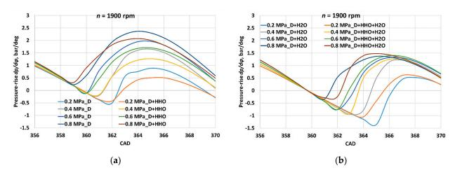
**Figure 14.** The pressure-rise  $dp/d\varphi$  vs. CAD for D and D+HHO modes (**a**), D+H<sub>2</sub>O and D+HHO+H<sub>2</sub>O modes at the various *BMEP* values (**b**).
