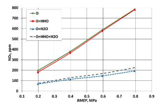
Figure 6. NO<sub>x</sub> emissions vs. BMEP with various fuel mixtures (and water injection).
