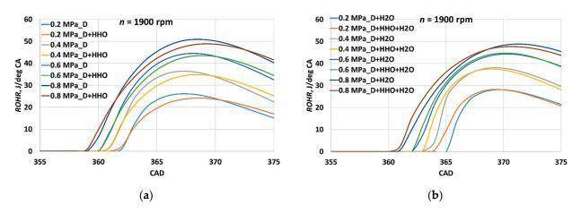
Figure 15. The *ROHR* vs. CAD for D and D+HHO modes (a), D+H<sub>2</sub>O and D+HHO+H<sub>2</sub>O modes at the various *BMEP* values (b).
