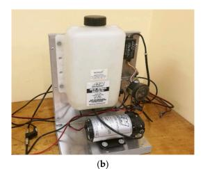
Figure 2. The water electrolyser (a) and AEM water injection kit with a pressure pump (b).
